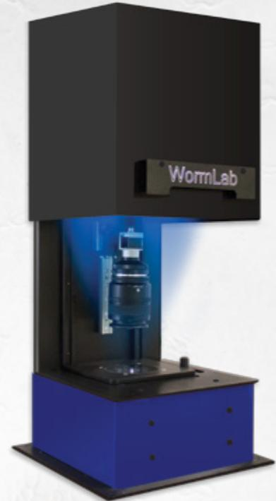
WormLab is a complete hardware and software solution for imaging and analyzing *C. elegans* behavior. Developed in collaboration with world-leading *C. elegans* researchers, it combines an intuitive worm tracking system with comprehensive analysis software.
